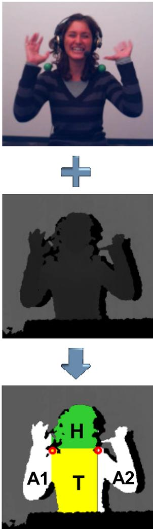
**Figure 1:** Input RGB and depth images are pre-processed to isolate user's head, trunk, arms and to track shoulder's markers.
