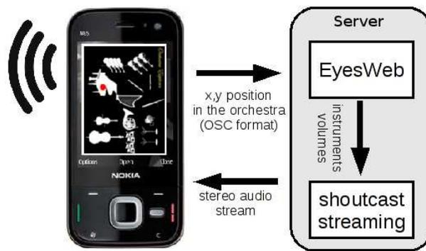
**Figure 2:** Mobile Orchestra Explorer architecture when audio rendering is sent back to the mobile phone: user moves in the orchestra space by tilting the mobile phone; user position is sent to Max/MSP for audio generation and audio is sent back in real-time to the user mobile phone.
