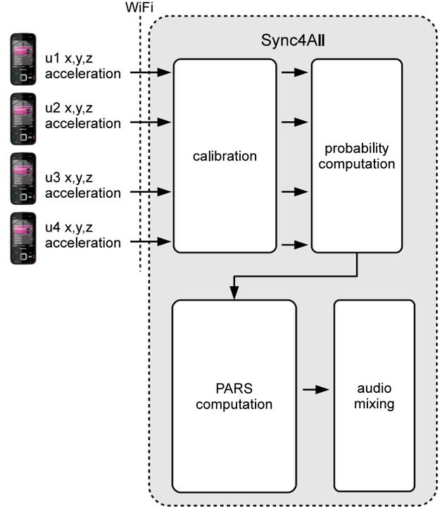
**Figure 1: The architecture of Sync4All. Acceleration data from mobile phones is processed to compute synchronisation between each pair of users. Synchronisation controls audio mixing.**
