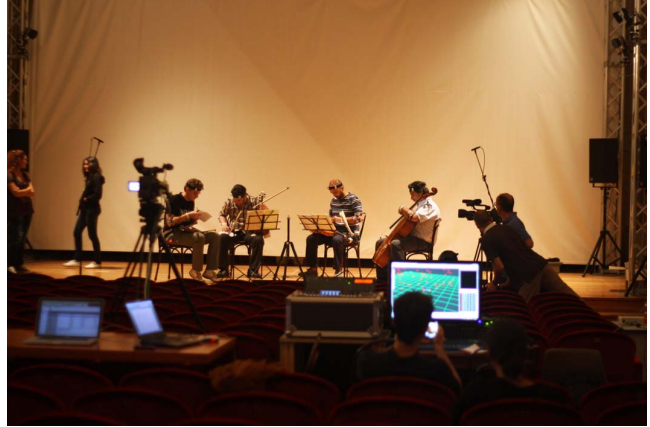
Fig. 1. The multimodal setup for the experiment : (a) motion capture, (b) videocamera (d) environmental microphones. Each musician wears markers for motion capture. Piezoelectric microphones are in the body of the instrument. Note the position of the SQ ear represented by the optical reflector placed on the tripod situated in the center of the quartet, at equal distance from each musician.
